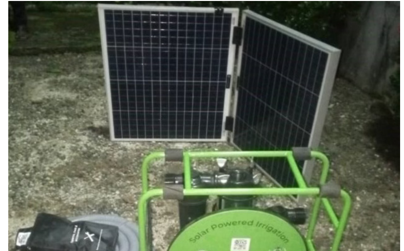
i Deployment of solar-powered irrigation pumps in Bayelsa State
