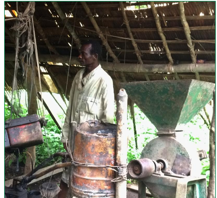
Local farmers use diesel generators to run machines that process palm oil, cassava/gari, and other crops
